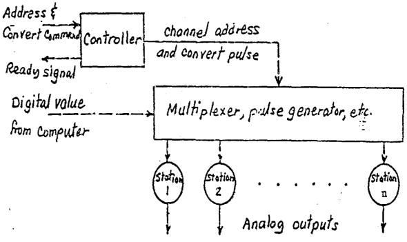
For the first type the computer must output the desired value of the signal, while for the second the computer output is the change in the signal.
